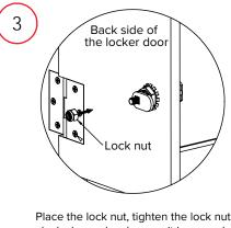
Place the lock nut, tighten the lock nut clockwise and make sure it is securely fastened but not too tight.
