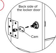
Insert the cam through the cylinder bolt and make sure the cam is facing towards the edge of the door.
