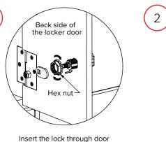
Insert the lock through door routing followed by the hex nut. Tighten the hex nut clockwise and make sure it is securely fastened.
